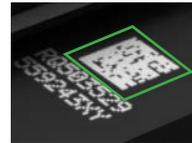
In-line cameras and sensors can be fix-mounted to meet the environmental conditions, protect against electrostatic discharge and even verify the bar codes.
